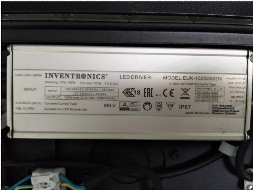
Figure 6 (Label of the LED driver)
