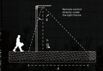
Remote control distance 5-8 meters, installation height and environment and other factors will affect the controller sensitivity, please refer to the actual field.
