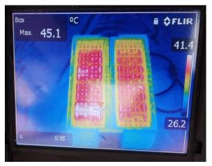
Temperature measurement point on TMP<sub>LED</sub>
