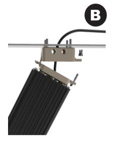
Step 2 - Attach the lamp body to the top of the junction box under the lid of the junction box. (Figure B)
