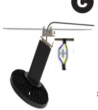
Step 3 - Connect the L,N,GND wires on the lamp to the corresponding L,N,GND cables on the pole. (Figure C)
