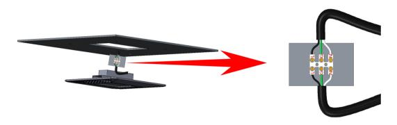
Step2: Wiring, connect the L,N,GND wires on the lamp to the corresponding L,N,GND cables on the pole.
