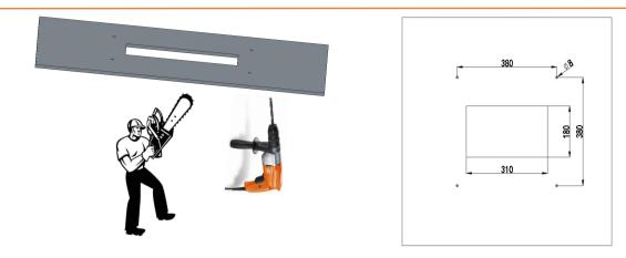
Step1: Use a chainsaw and an electric drill to make holes in the ceiling, the dimensions are as shown
