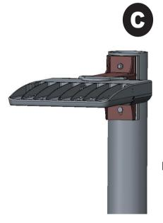
Step 3 - Fix the LED on the stand adapter and secure with the M8 screw (Figure C)
