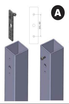
Step 1 - Install the back plate inside the pole with top bolt,
