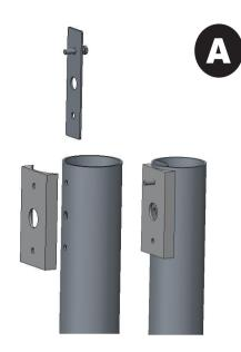
Step 1-Install the backplane and bracket adapter on the pole with top bolts, nuts and washers (Figure A)
